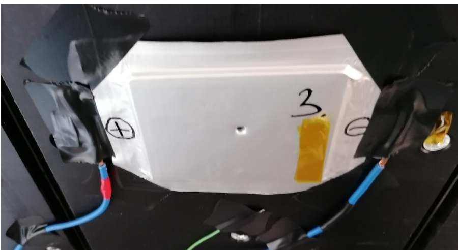
Picture 9 DUT after nail penetration test (after removal of nail)
